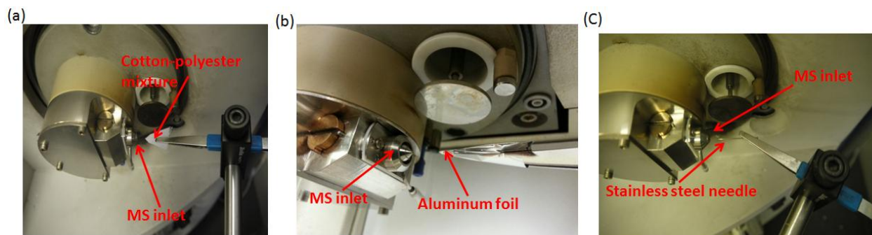
Figure 2. ESI source with (a) cotton-polyester mixture, (b) aluminum foil and (c) stainless steel needle as sample loading solid substrate.
